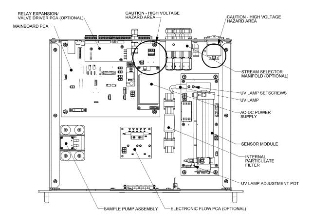
Figure 9-1: Instrument Layout, Rack Mount Configuration
